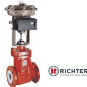
RICHTER bellows-sealed globe control valve - PFA lining DN 15 to DN 100
