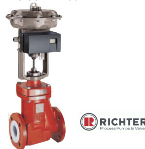
RICHTER bellows-sealed globe control valve - PFA lining DN 15 to DN 100
